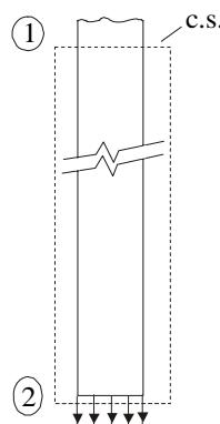
$$\frac{p_1}{\gamma} + \frac{V_1^2}{2g} + z_1 = \frac{p_2}{\gamma} + \frac{V_2^2}{2g} + z_2 + h_L$$
