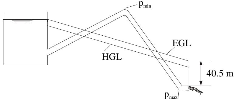
Minimum pressure. Apply the Energy equation (point 1 on reservoir surface; point 2 in pipe at location of minimum pressure)
