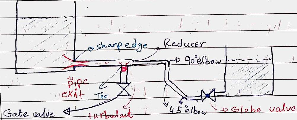
for tank exit or pipe inlet
