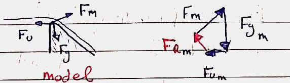
$$* \text{inertitic forces} = \frac{\gamma_m L_m^3 a_m}{\gamma_p L_p^3 a_p} = \frac{\rho_m L_m^3 (U_m / t_m)}{\rho_p L_p^3 (U_p / t_p)}$$
