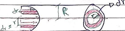
$$\bar{V} = \frac{\int_0^R V_{\max} \left(1 - \frac{r^2}{R^2}\right) 2\pi r dr}{\pi R^2}$$
