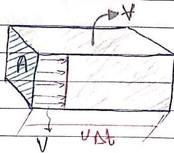
$$\frac{\Delta V}{\Delta t} = Q \quad (\text{Volumetric flow rate}) \text{ m}^3/\text{s}$$
