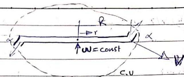
steady  $\rightarrow \frac{d}{dt} \int_{c.v.} (\vec{r} \times \vec{v}) \rho dV = 0$
