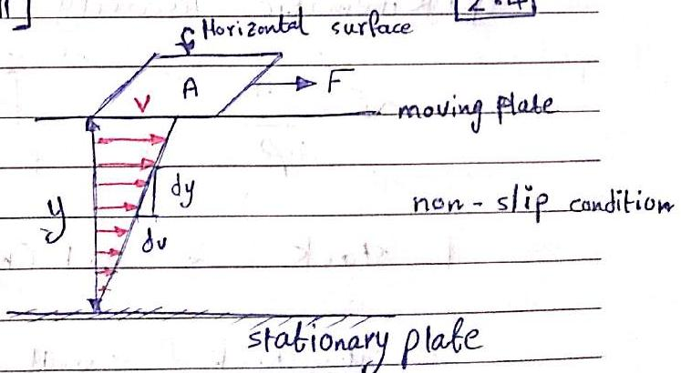
$$\text{But } T \text{ (shear stress)} = \frac{F}{A}$$
