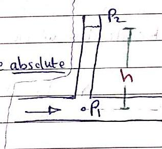
$$P_1 = \rho g h \quad P_2 = P_{atm} = 0 \quad (\text{in gage measuring})$$
