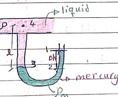
② Pressure is the same in the same liquid in same elevation.  $P_2 = P_3 \quad \dots \quad ②$
