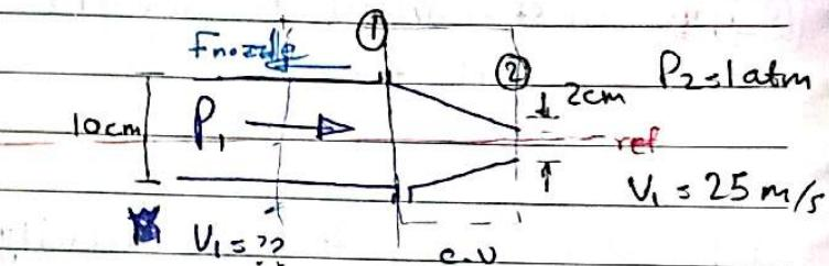
$$P_1 = P_2 - \rho \frac{(V_2^2 - V_1^2)}{2} \rightarrow P_1 = 311.2 \text{ kPa gage}$$
