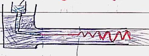
if  $\frac{PUD}{\mu} > 2000$  and  $< 3000 \rightarrow$  Transition. laminar turbulentif  $\frac{PUD}{\mu} > 3000 \rightarrow$  Turbulent.
