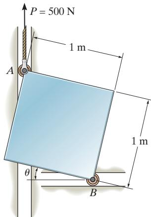
$$T_2 = \frac{1}{2} m(v_G)_2^2 + \frac{1}{2} I_G \omega_2^2$$
