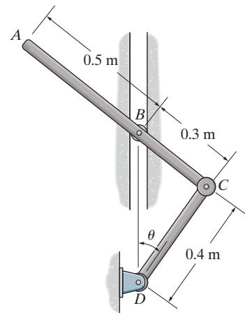
$$V_1 = (V_g)_1 = W_1(y_{G1})_1 + W_2(y_{G2})_1 \\ = 6(9.81)(0.8) + 3(9.81)(0.2) = 52.974 \text{ J}$$
