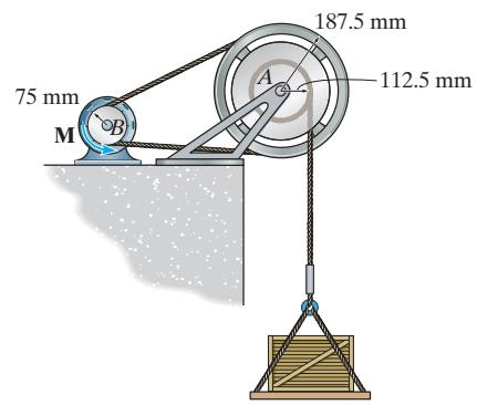
$$\begin{aligned} T &= T_A + T_C \\ &= \frac{1}{2} I_A \omega^2 + \frac{1}{2} m_C v_C^2 \\ &= \frac{1}{2} (0.5625) \omega^2 + \frac{1}{2} (100) [\omega(0.1125)]^2 \\ &= 0.91406 \omega^2 \end{aligned}$$
