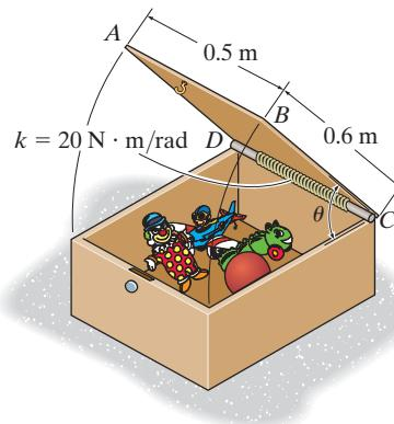
**Kinetic Energy and Work:** Since the cover rotates about a fixed axis passing through point C, the kinetic energy of the cover can be obtained by applying  $T = \frac{1}{2} I_C \omega^2$ , where  $I_C = \frac{1}{3} mb^2 = \frac{1}{3}(6)(0.6^2) = 0.72 \text{ kg} \cdot \text{m}^2$ . Thus,
