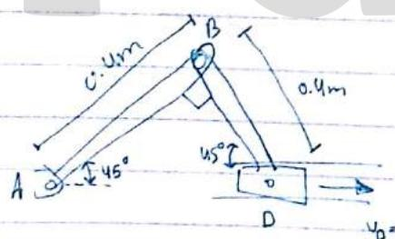
$$\omega_{AB} = ? \quad \omega_{BD} = \frac{v_B}{r_{B/Ic}} = \frac{3}{0.4/\cos 45^\circ} = ?$$
