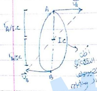
$$\omega = \frac{\omega_A}{r_{A/Ic}} = \frac{\omega_B}{r_{B/Ic}}$$
