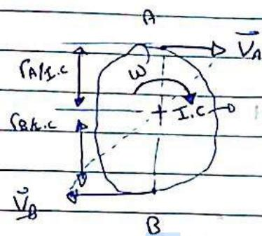
$$\omega = \frac{V_A}{r_{A/I.C}} = \frac{V_B}{r_{B/I.C}}$$
