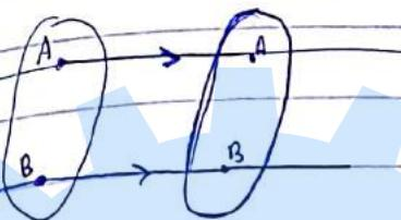
Rectilinear motion (straight path + the points don't move, orientation of A/B is const.)
