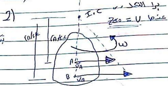
$$\omega = \frac{V_A}{r_{A/I.C}} = \frac{V_B}{r_{B/I.C}}$$
