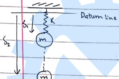
$$V_1 = V_g + V_{ei} = -ws_1 + \frac{1}{2} ks_1^2$$
