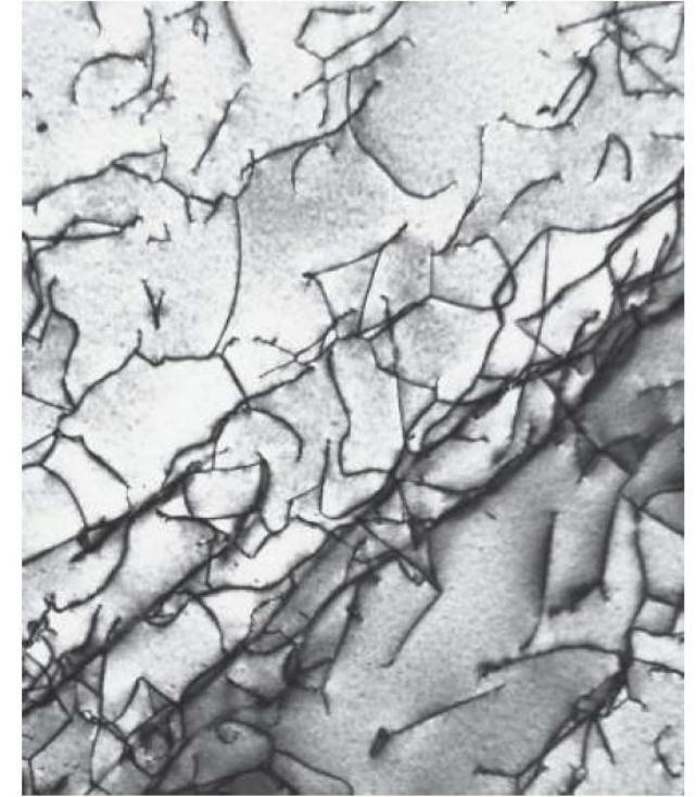
A transmission electron micrograph of a titanium alloy in which the dark lines are dislocations, 50,000 \times .
