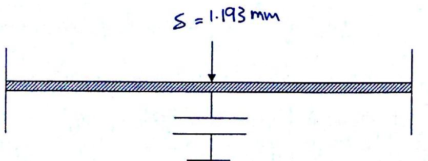
→ after  $\therefore d = 3.5 \text{ mm} - 1.193 \text{ mm} = 2.307 \text{ mm}$
