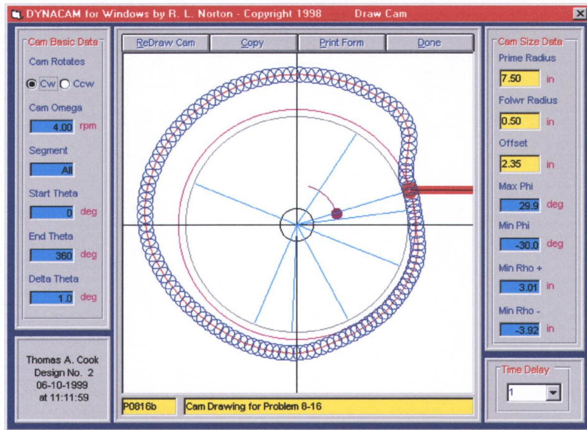
4. The minimum and maximum pressure angles and radius of curvature are shown in the figure above. The design has the following dimensions:
