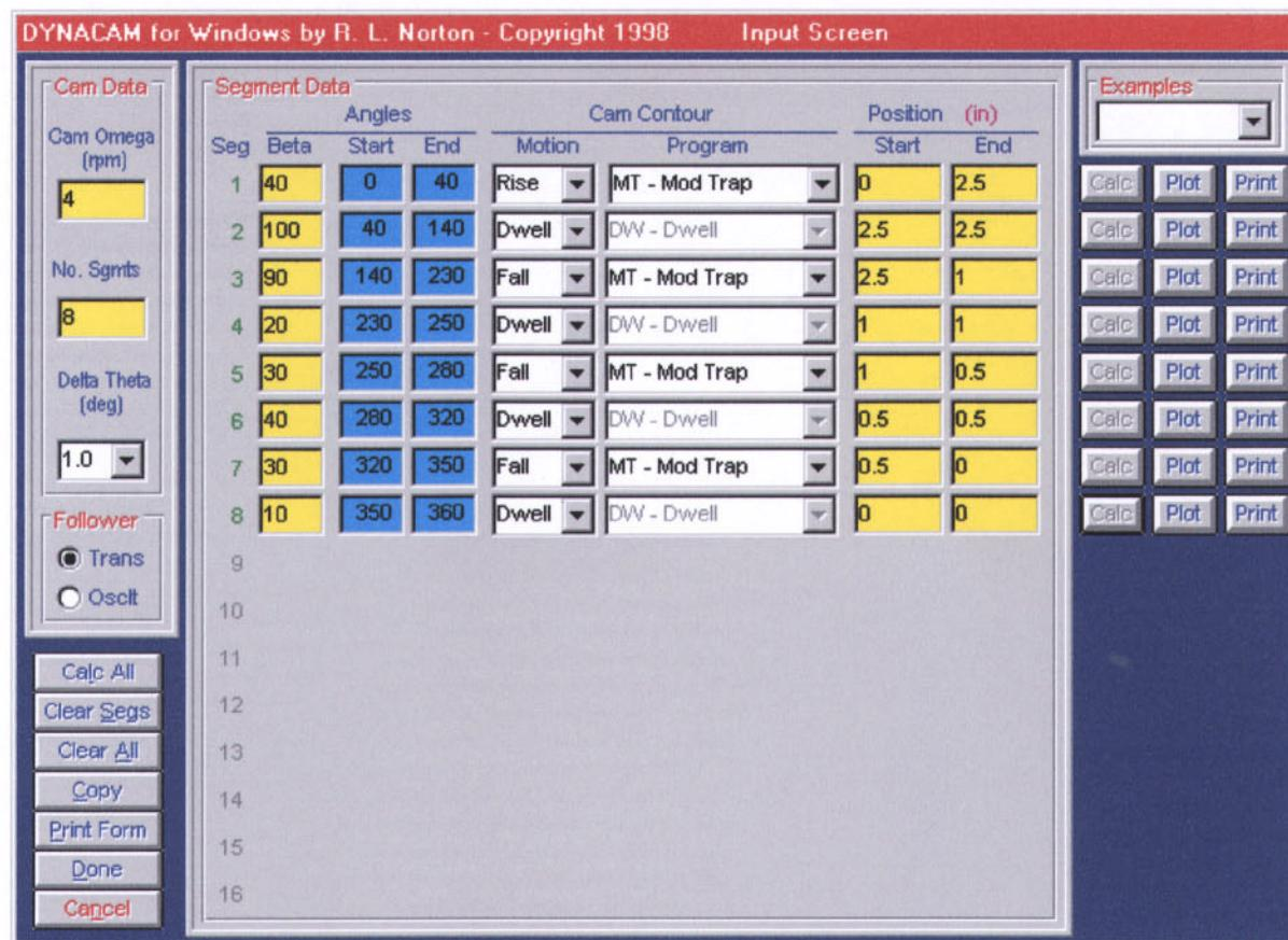
3. The cam was sized iteratively to balance the positive and negative extreme values of the pressure angle by varying the eccentricity and to reduce the maximum absolute pressure angle to 30 deg or less by increasing the prime circle radius. The resulting cam is shown below.
