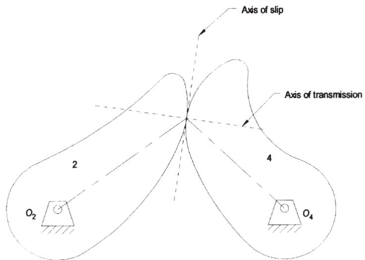
2. As defined in Section 8.6 and Figure 8-41, the pressure angle is the angle between the direction of motion of the follower and the direction of the axis of transmission. Establish those two directions and measure the angle between them.
