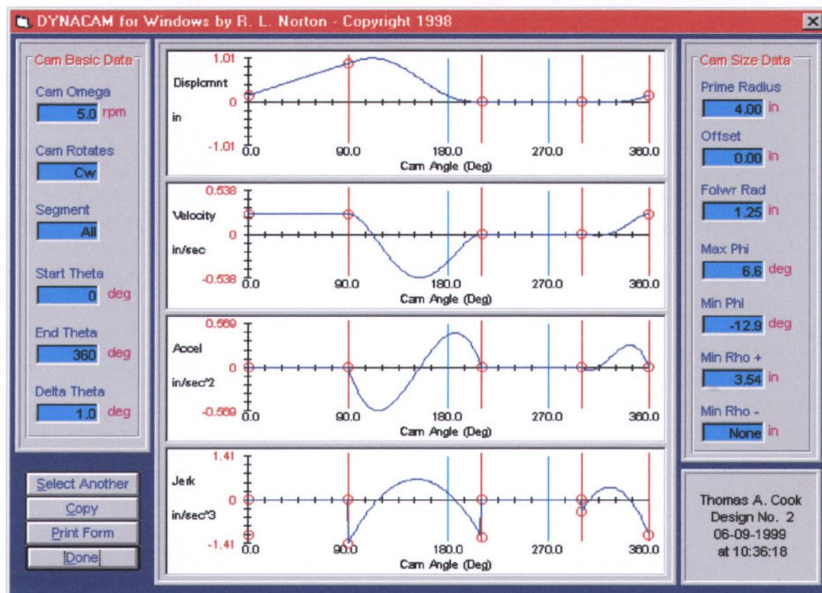
8. From *SVAJ* diagrams we see that all design goals are met but the peak acceleration in segment 2 is higher than the peak in segment 4. These can be more evenly balanced by increasing the segment 2 interval and decreasing the segment 4 interval. Iterate on these intervals until the peak accelerations are more nearly the same. Note also that  $\rho_{min}$  is not greater than 3 times  $R_f$
