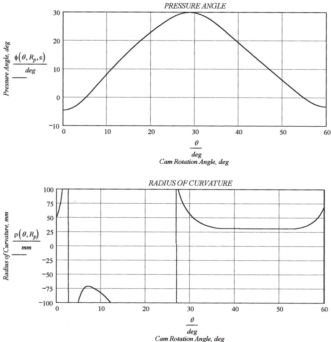
7. The graphs above show the pressure angle and radius of curvature for the values of  $R_p$  and  $\epsilon$  entered on the first page. These values will be iterated below to obtain a balanced pressure angle whose absolute value is not greater than 20 deg.
