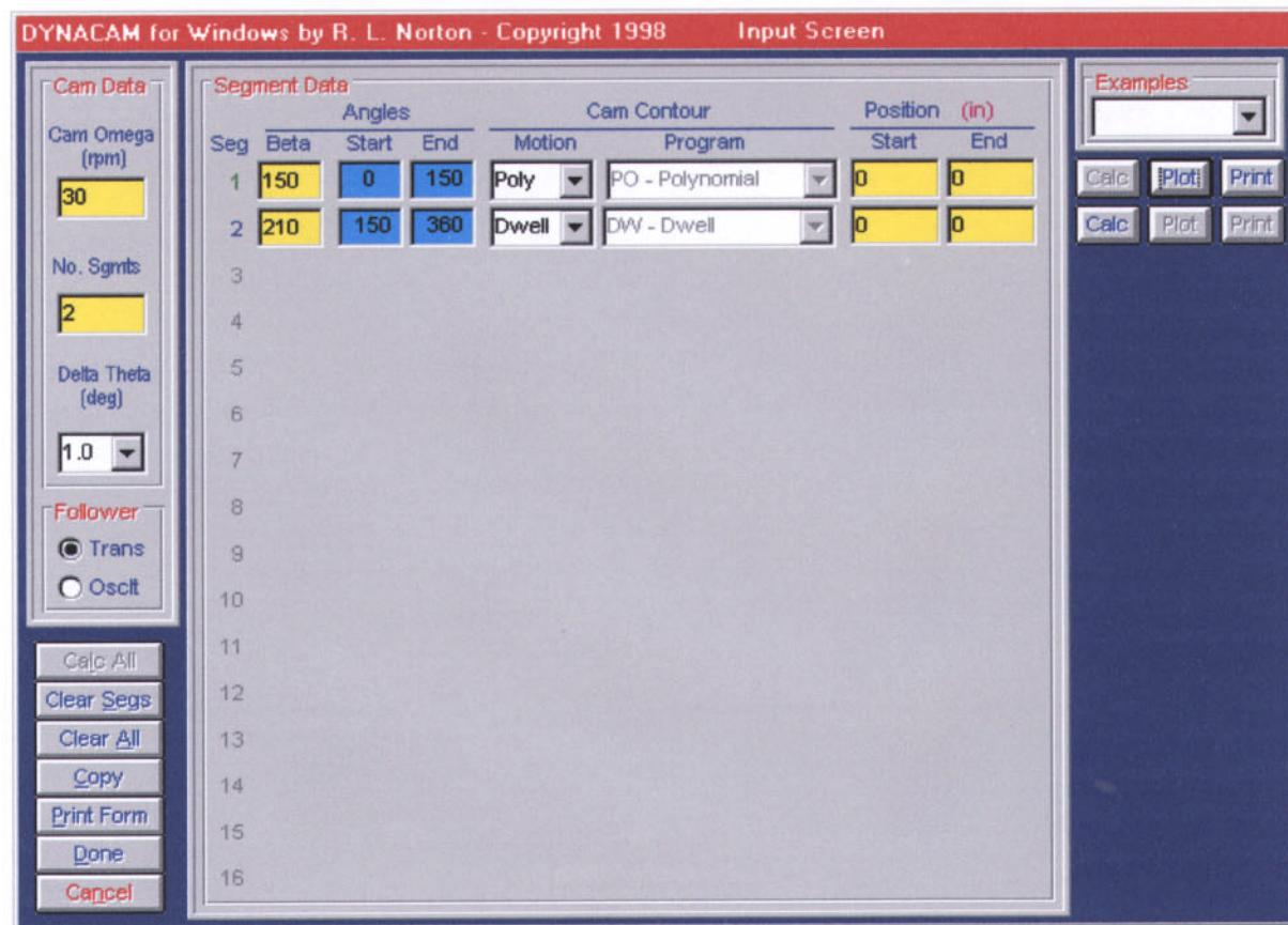
3. The cam was sized iteratively to balance the positive and negative extreme values of the pressure angle by varying the eccentricity and to reduce the maximum absolute pressure angle to 30 deg or less by increasing the prime circle radius. The resulting cam is shown below.
