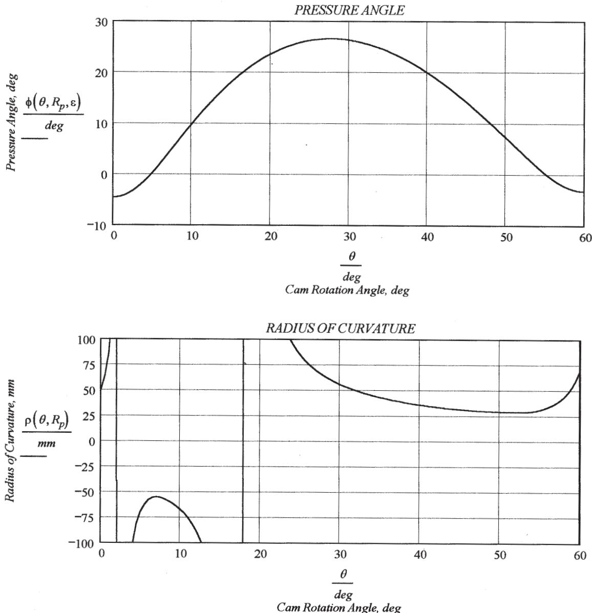
7. The graphs above show the pressure angle and radius of curvature for the values of  $R_p$  and  $\varepsilon$  entered on the first page. These values will be iterated below to obtain a balanced pressure angle whose absolute value is not greater than 20 deg.
