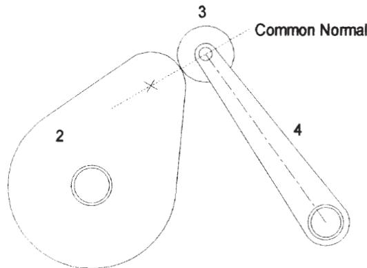
2. As described in Section 8.1 and Figure 8-1, find the centers of curvature of the cams, which are located on the common normal (axis of transmission). They will be the locations of the moving pivots of the effective pin-jointed fourbar linkage.
