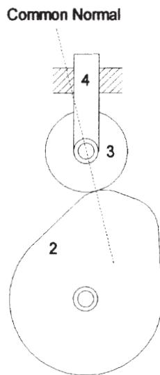
2. As described in Section 8.1 and Figure 8-1, find the centers of curvature of the cams, which are located on the common normal (axis of transmission). They will be the locations of the moving pivots of the effective pin-jointed fourbar linkage.
