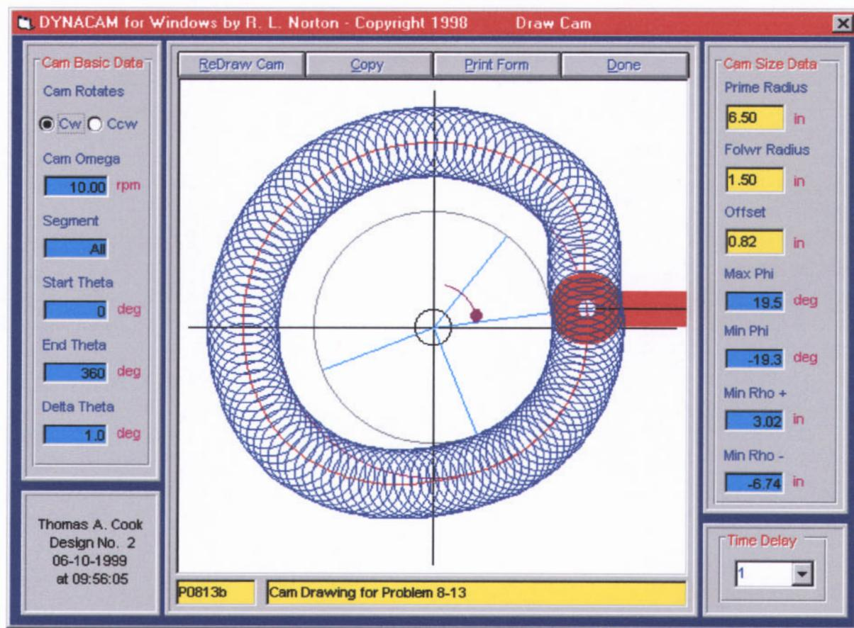
4. The minimum and maximum pressure angles and radius of curvature are shown in the figure above. The prime radius had to be increased above that which was necessary for the pressure angle constraint in order to provide a minimum radius of curvature that was twice the roller follower radius. The design has the following dimensions:
