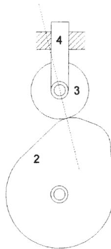
2. As defined in Section 8.6 and Figure 8-41, the pressure angle is the angle between the direction of motion of the follower and the direction of the axis of transmission. Establish those two directions and measure the angle between them.
