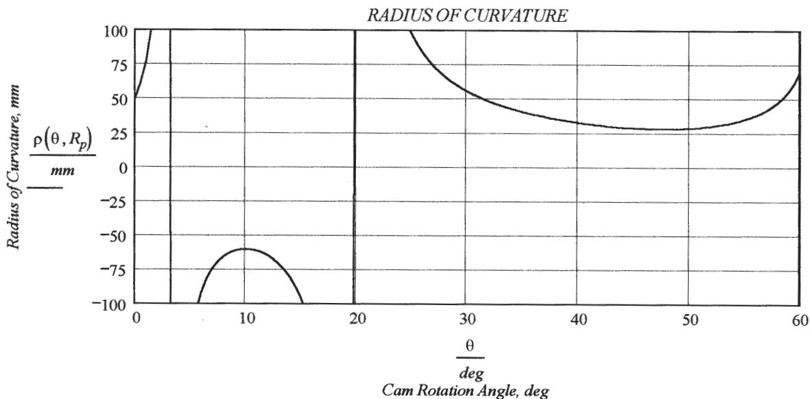
4. The graphs above show the pressure angle and radius of curvature for the values of  $R_p$  and  $\epsilon$  entered on the first page. These values will be iterated below to obtain a balanced pressure angle whose absolute value is not greater than 20 deg.
