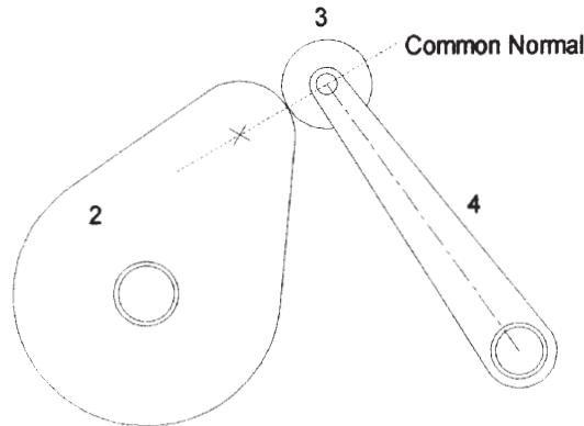
2. As defined in Section 8.6 and Figure 8-41, the pressure angle is the angle between the direction of motion of the follower and the direction of the axis of transmission. Establish those two directions and measure the angle between them.
