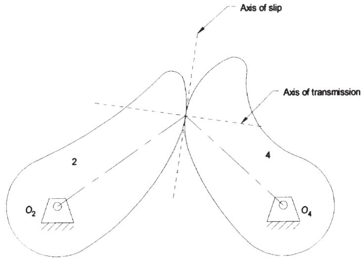
2. As described in Section 8.1 and Figure 8-1, find the centers of curvature of the cams, which are located on the common normal (axis of transmission). They will be the locations of the moving pivots of the effective pin-jointed fourbar linkage.
