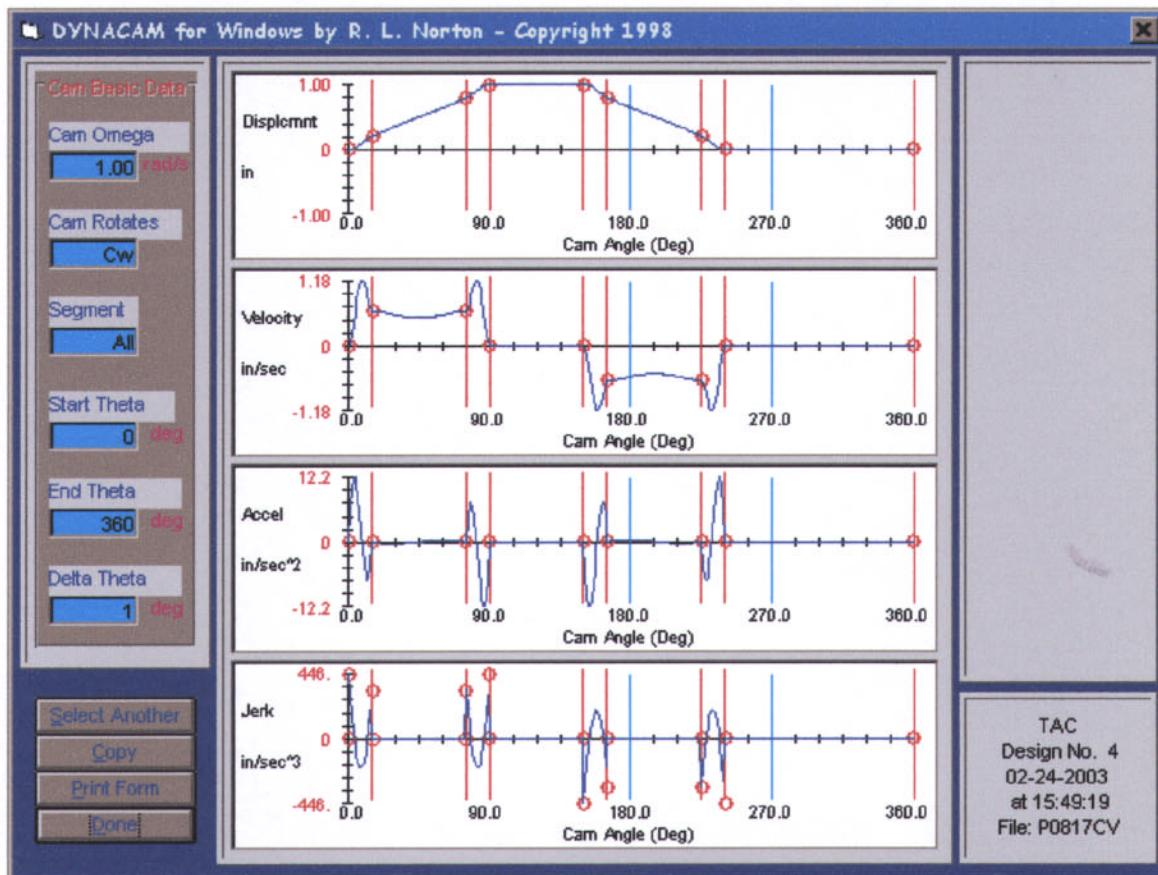
1. The DYNACAM output screen for the modified sine profile is shown below. The maximum acceleration and jerk are 74.4 and 105, respectively. Obviously, for the CV-poly design choices that were made, the modified sine profile results in lower inertia forces and a smoother follower motion.
