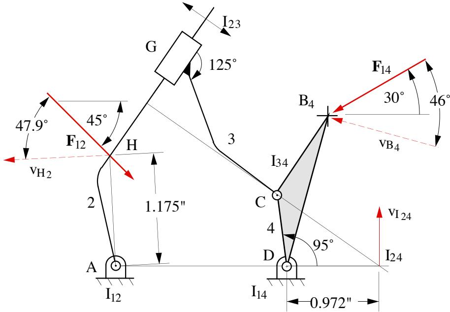
Assume that link 4 rotates CCW. Then  $\mathbf{v}_{I_{24}}$ ,  $\mathbf{v}_{B_4}$ , and  $\mathbf{v}_{H_2}$  will be in the directions shown above. From conservation of power,
