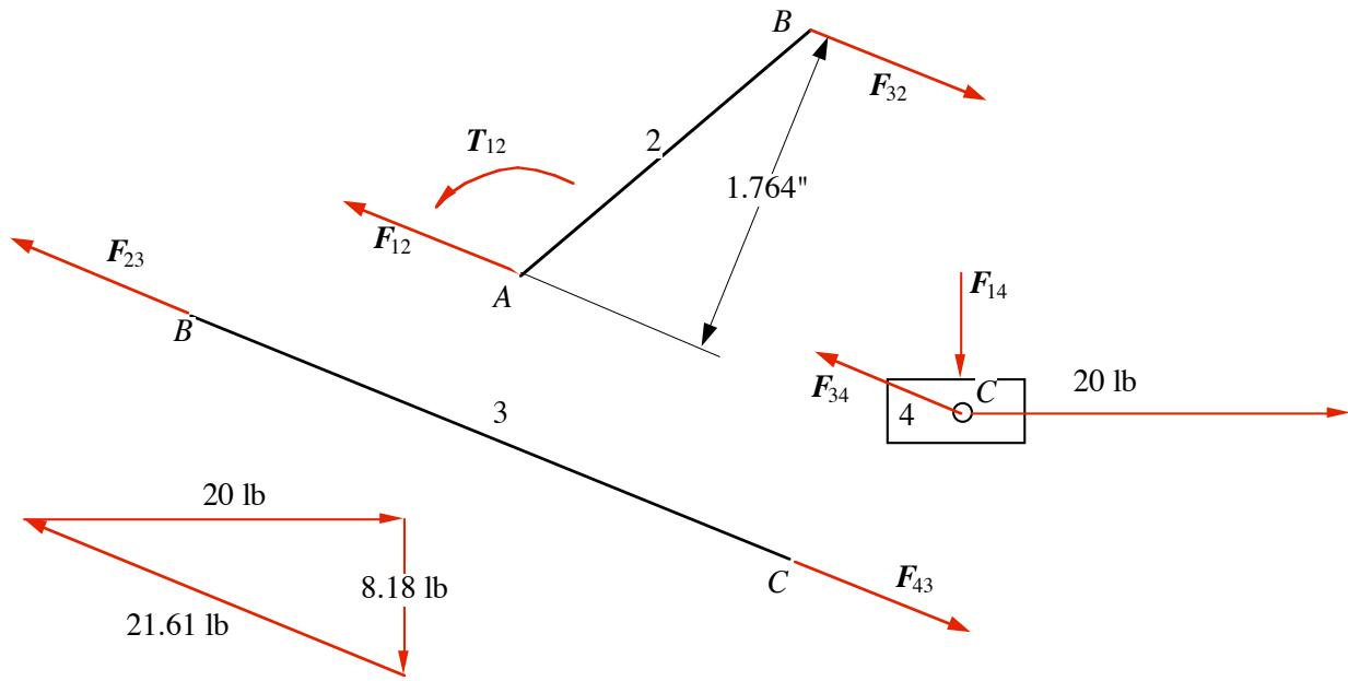
By summing forces vectorially on link 4, the magnitudes of all the forces can be determined. The force summation equation is
