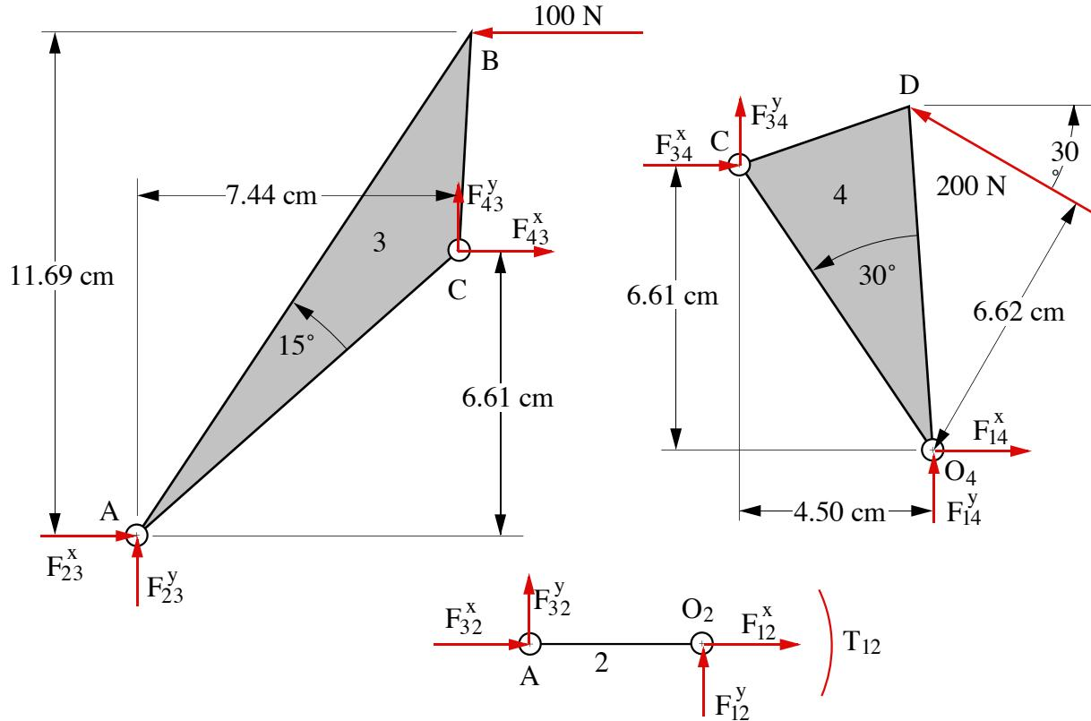
For the freebody diagram for link 4, assume initially that all of the unknown forces are in the positive x and y directions. Then a negative result will indicate that the forces are in the negative direction. Summing forces in the X and Y directions gives
