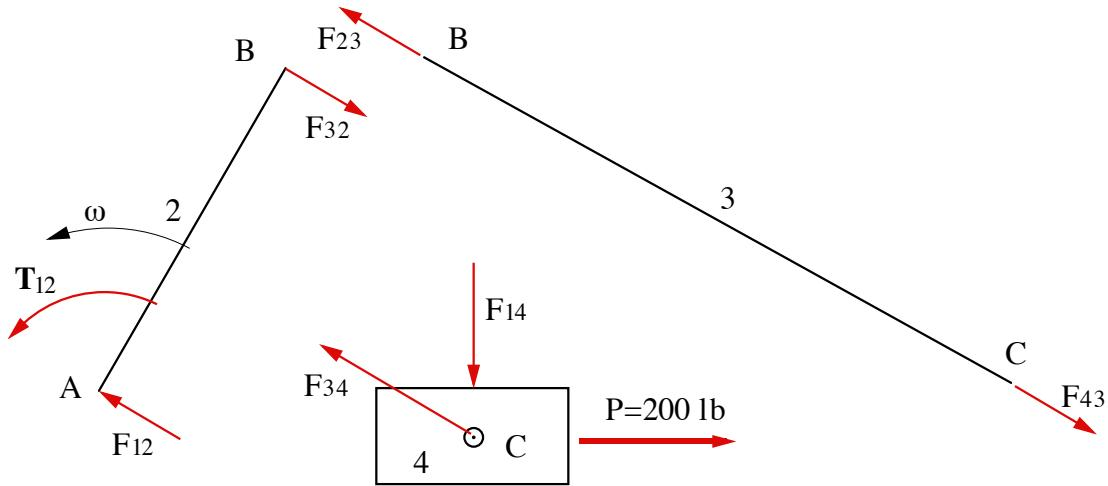
To analyze the system with friction, we need to compute the friction angle and friction circle radius for each joint. The friction angle is
