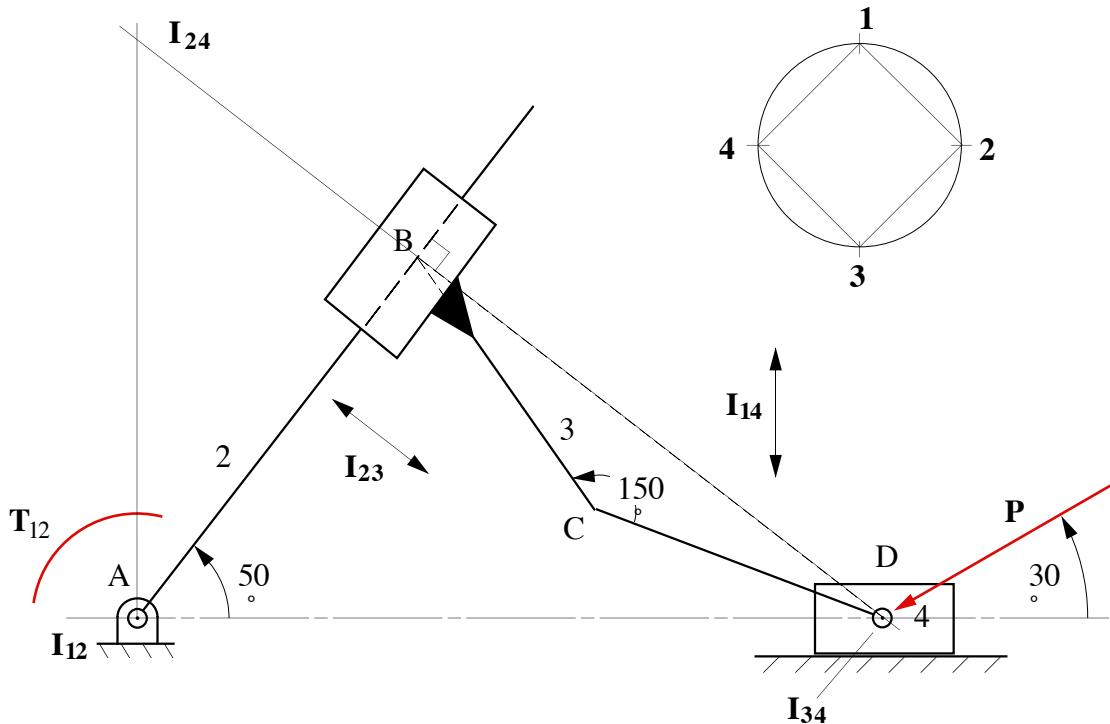
To determine the sign of  $T_{12}$ , assume that the angular velocity of link 2 is counter-clockwise. Then the velocity of  $D_4$  will be generally in the same direction as the force  $P$  and power will be taken out of the system at link 4. Therefore, power will be taken out of the system at link 2, and the torque  $T_{12}$  must be clockwise.
