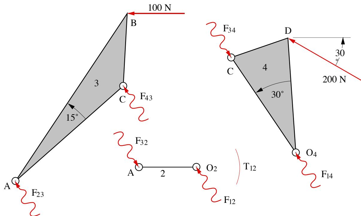
The freebody diagram of each link is shown above. From the freebody diagrams, it is clear that no single free body can be analyzed separately because in each case, four unknowns result. Therefore, we must write the equilibrium equations for each freebody, and solve the equations as a set.
