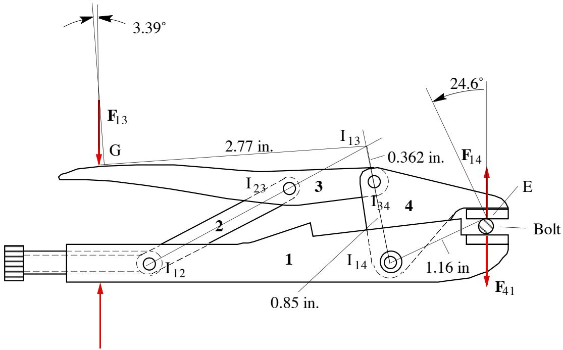
$${}^1V_{B4} = {}^1\omega_4 \times r_E / I_{14}$$
