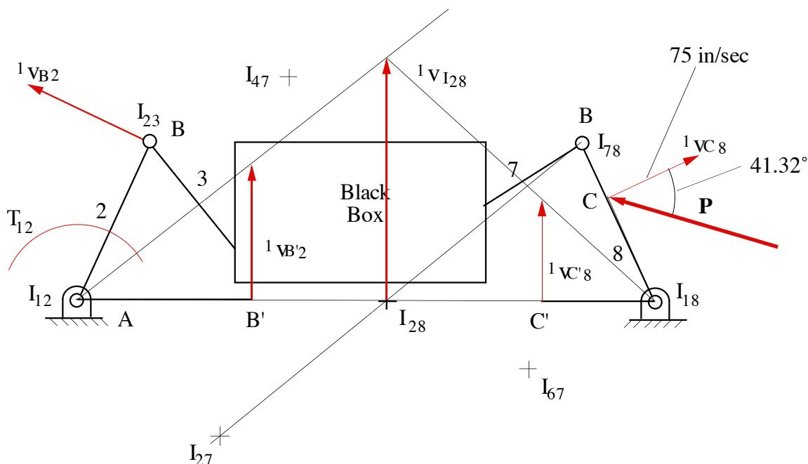
Find instant centers  $I_{12}$ ,  $I_{18}$ , and  $I_{28}$ . Then use the rotating radius method to find the velocity of C8. The results are shown on the figure. From the figure,
