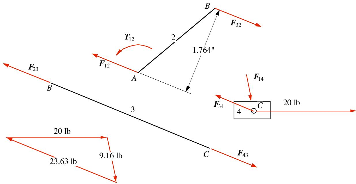
By summing forces vectorially on link 4, the magnitudes of all the forces can be determined. The force summation equation is
