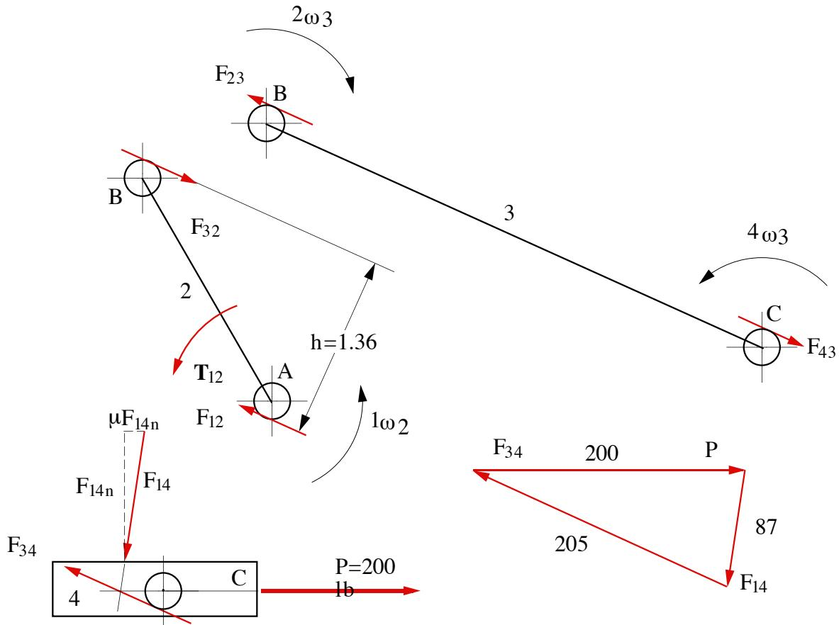
By summing forces vectorially on link 4, the magnitudes of all the forces can be determined. The force summation equation is
