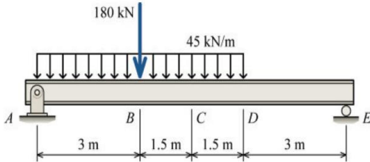
$$\Delta_C = \frac{5,223.868 \text{ kN}\cdot\text{m}^3}{EI} = \frac{5,223.868 \text{ kN}\cdot\text{m}^3}{3.4 \times 10^5 \text{ kN}\cdot\text{m}^2}$$
