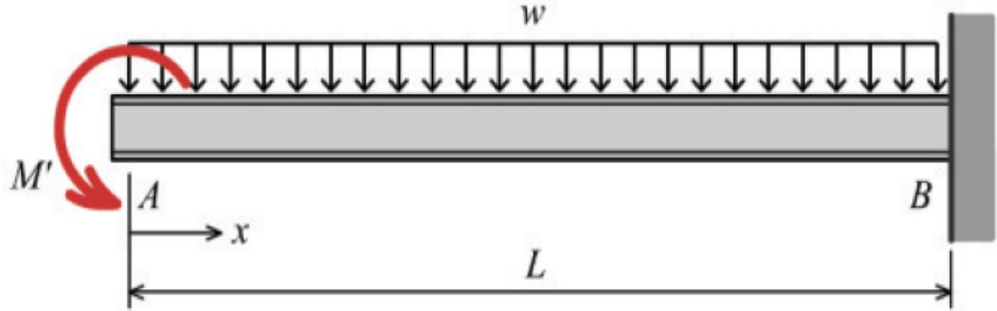
$$\theta = \int_0^L \left( \frac{\partial M}{\partial M'} \right) \frac{M}{EI} dx = \int_0^L -1 \left( -\frac{wx^2}{2EI} \right) dx = \int_0^L \frac{wx^2}{2EI} dx$$
