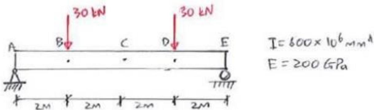
Calculate the vertical displacement of point C ( $\Delta_C \downarrow$ ) using Castigliano's theorem. Neglect the strain energy due to shear.
