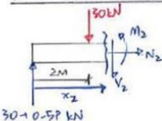
$$[+] \sum M_C = 0 \quad M_2 - [(30 + 0.5P)kN] \times x_2 + [30 \text{ kN} \times (x_2 - 2)] = 0$$
