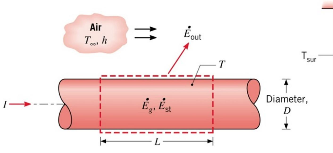
A long conducting rod of diameter  $D$  and electrical resistance per unit length  $R'_e$  is initially in thermal equilibrium with the ambient air and its surroundings. This equilibrium is disturbed when an electrical current  $I$  is passed through the rod. Develop an equation that could be used to compute the variation of the rod temperature with time during the passage of the current.
