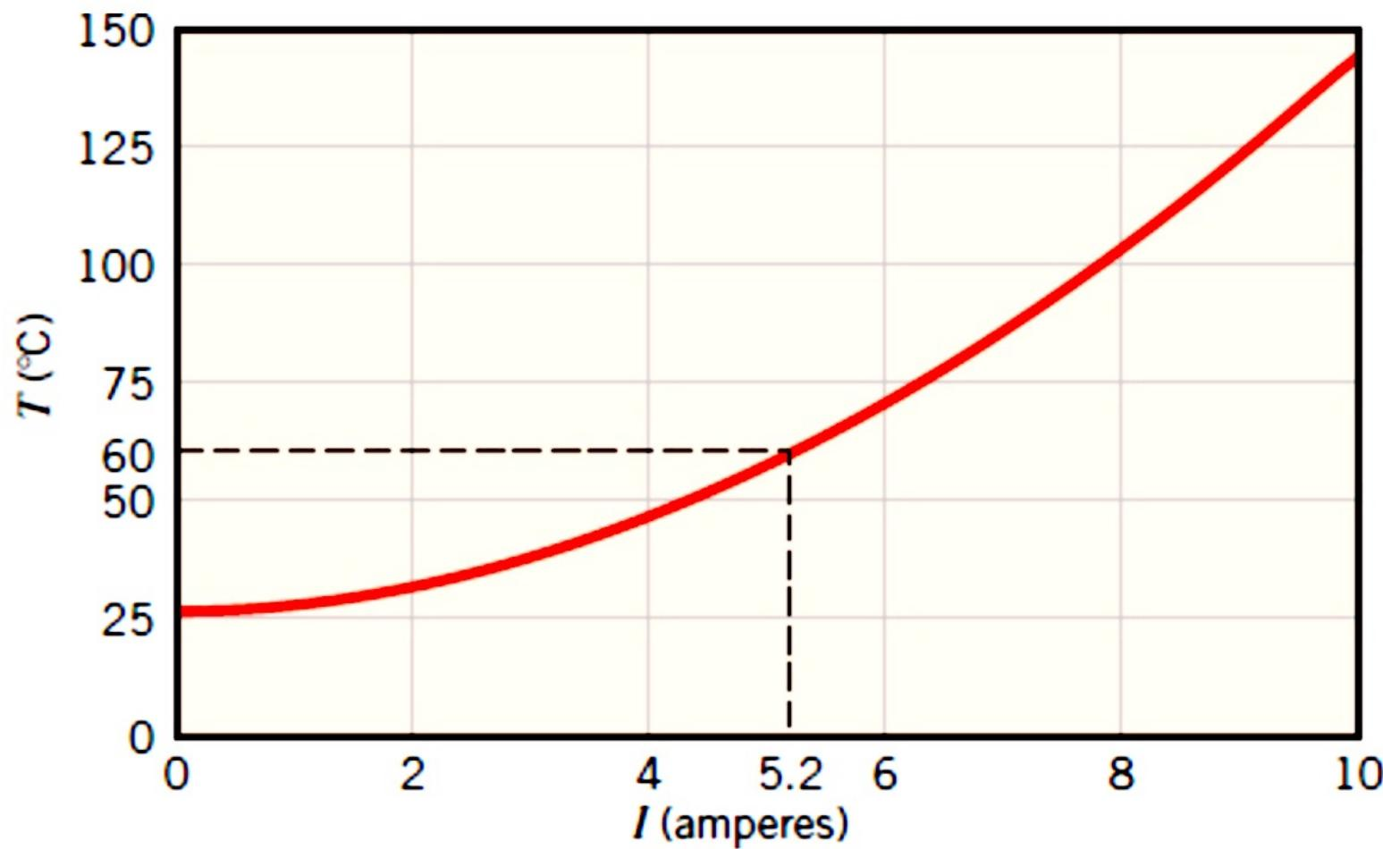
4. If a maximum operating temperature of  $T = 60^\circ\text{C}$  is prescribed for safety reasons, the current should not exceed 5.2 A.
