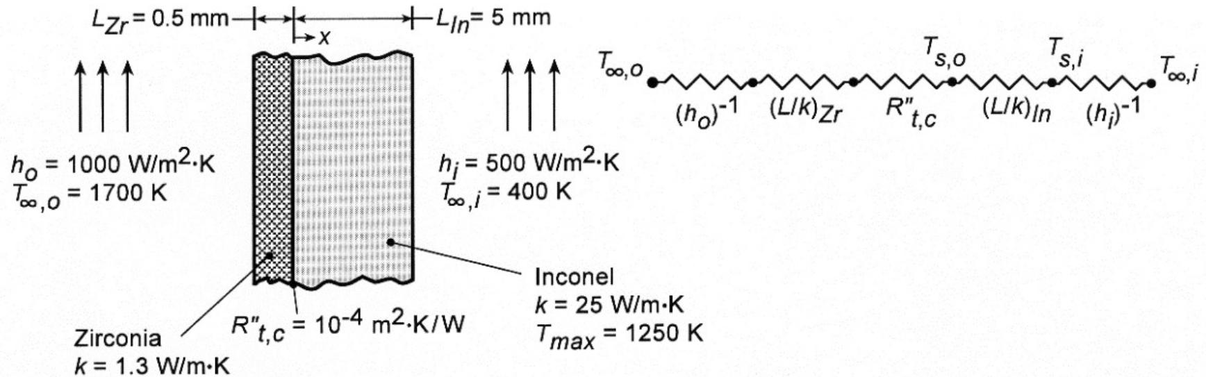
ASSUMPTIONS: (1) One-dimensional, steady-state conduction in a composite plane wall, (2) Constant properties, (3) Negligible radiation.
