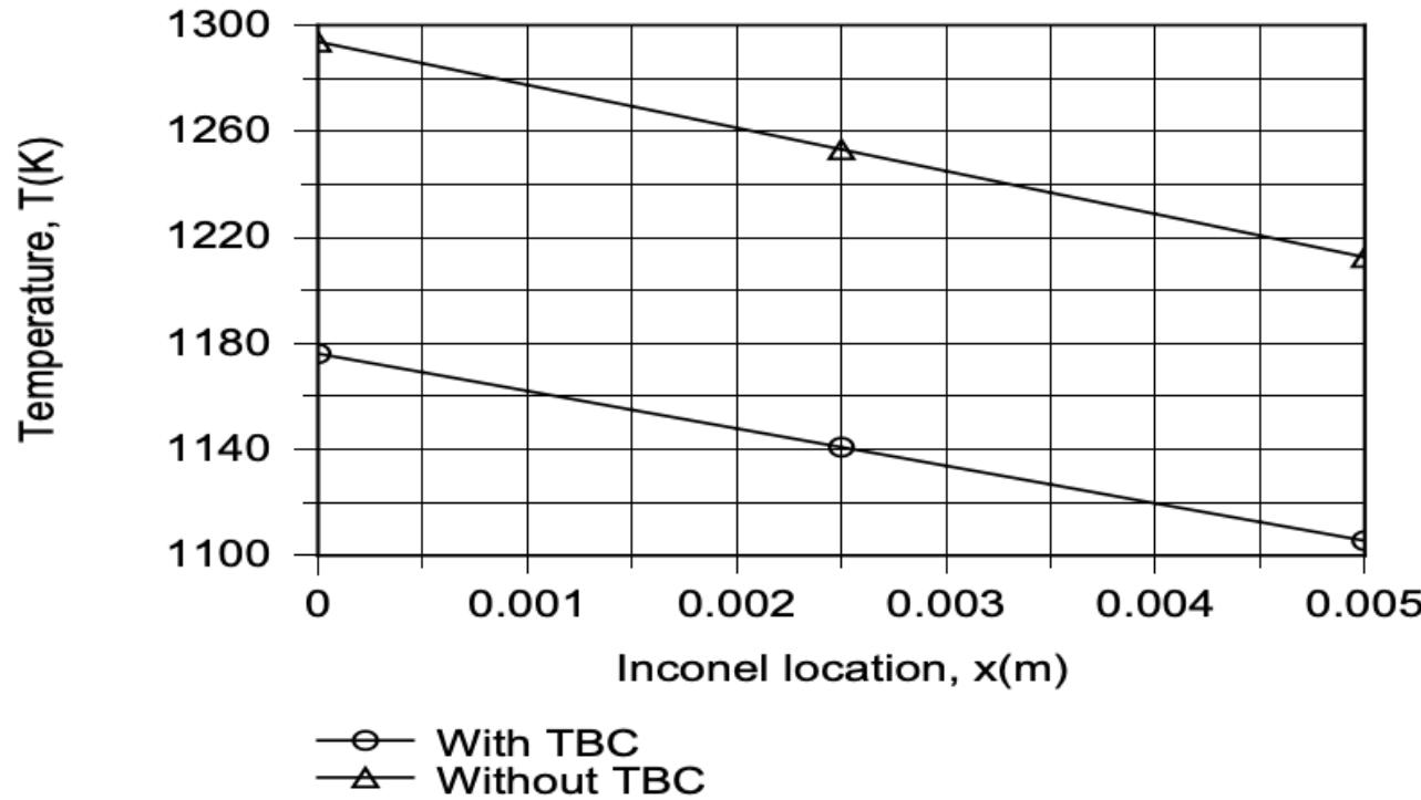
COMMENTS: Since the durability of the TBC decreases with increasing temperature, which increases with increasing thickness, limits to its thickness are associated with reliability considerations. In this application, thermal contact resistance is desirable.
