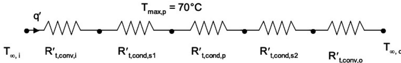
Equating the heat rate per unit length of tubing from the crude oil to the inner surface of the polyurethane with the heat rate from the inner surface of the polyurethane to the oceanic waters yields
