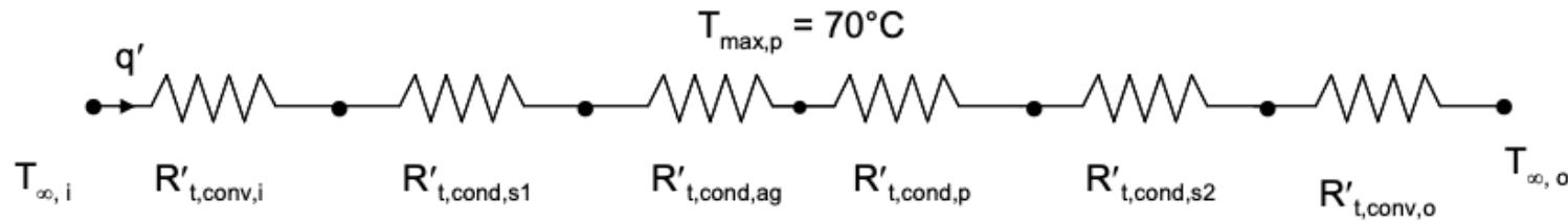
The thermal resistance values are as before, except the conduction resistance per unit length in the polyurethane is decreased, since its thickness is reduced relative to part (a). In addition, the conduction resistance for the aerogel must be evaluated. These two resistances are:
