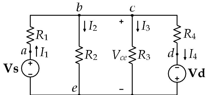
2. Set the DC supplies output voltage controls to minimum then connect them to the circuit. Switch both DC supplies ON, and set their voltages to  $V_s = 9$  Volts and  $V_d = 14$  Volts. Verify these voltages using a voltmeter.
