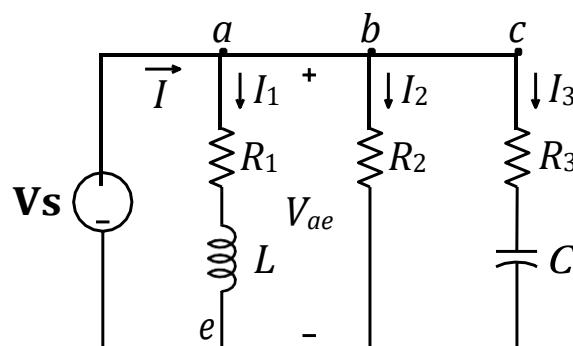
2. Set the DC supply output voltage controls to minimum then connect it to the circuit. Switch the DC supply ON, and set its voltage  $V_s$  to 9 Volts. Verify this voltage using a voltmeter.
