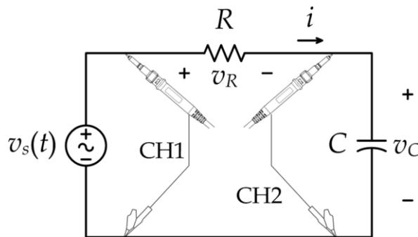
2. Set the function generator to produce a **sinusoidal** waveform (AC) with frequency of **50 Hz**, and peak to peak voltage of  **$V_{\text{pp}} = 10 \text{ V}$** .
