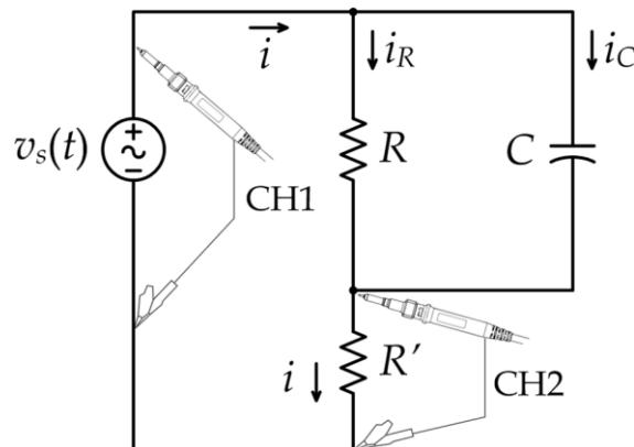
3. Use the oscilloscope to measure the **peak to peak** value of the voltage  $V_{R'}$  and its phase shift compared to  $V_s$ . Record the measurements in Table 4 in the report.
