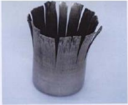
Deep drawn cup made from non-stable austenitic stainless steel. A number of cracks are after the deep drawing formed in the upper part of the cup due to residual stresses in the cup wall.
