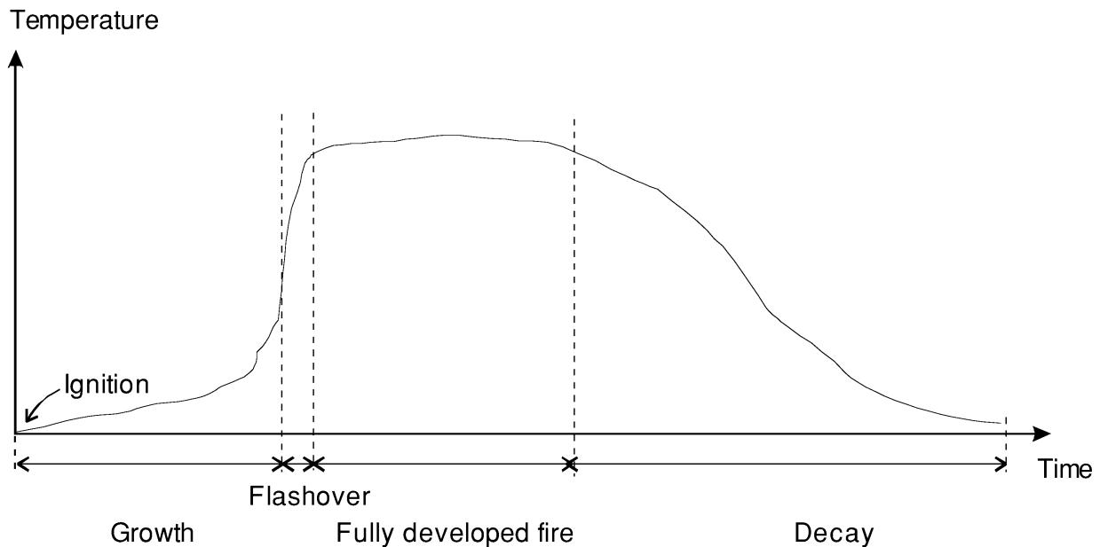
FIGURE 2.5 Idealized description of the temperature variation with time in an enclosure fire.
