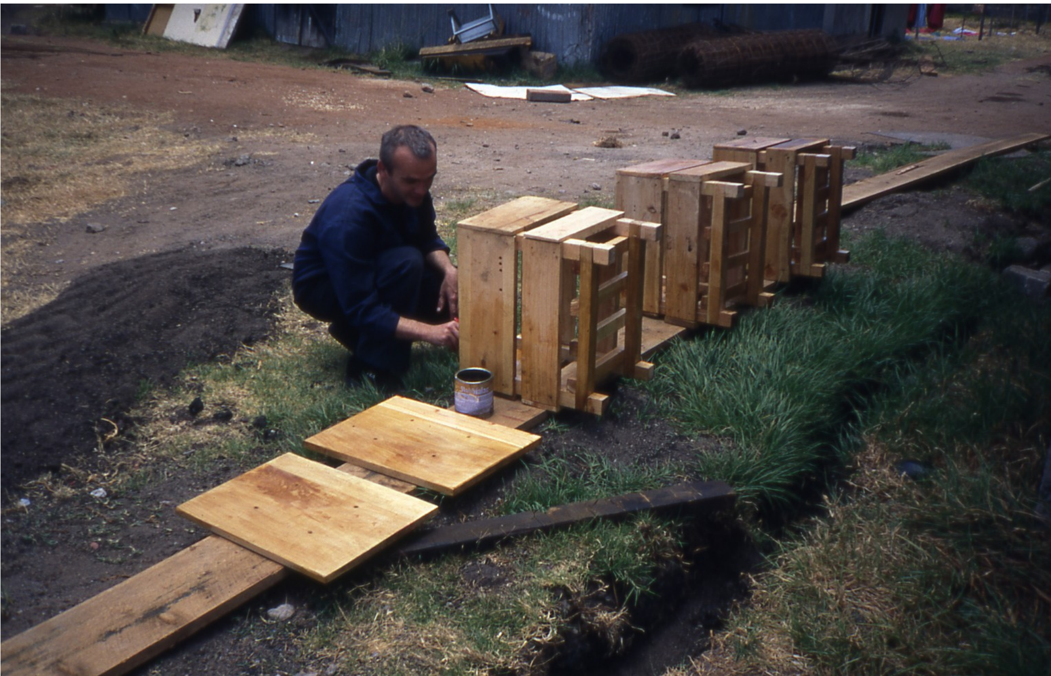
Battery boxes for staff solar systems, Wasso Hospital, Tanzania
