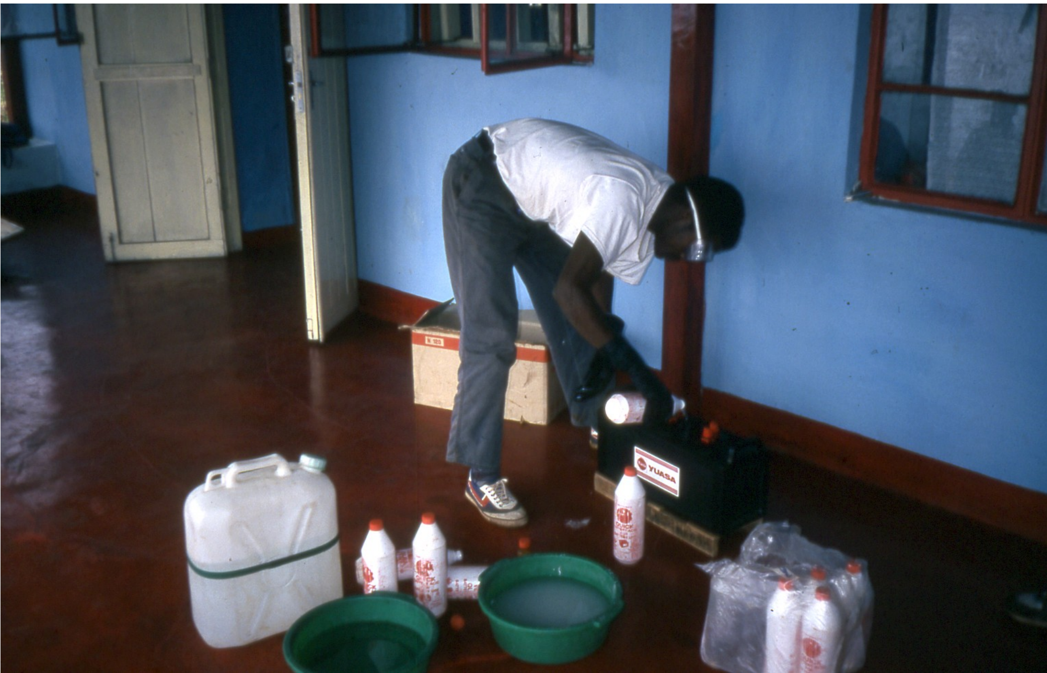
Azaria putting acid in new batteries – note goggles, gloves, bowls of water, Tanzania
