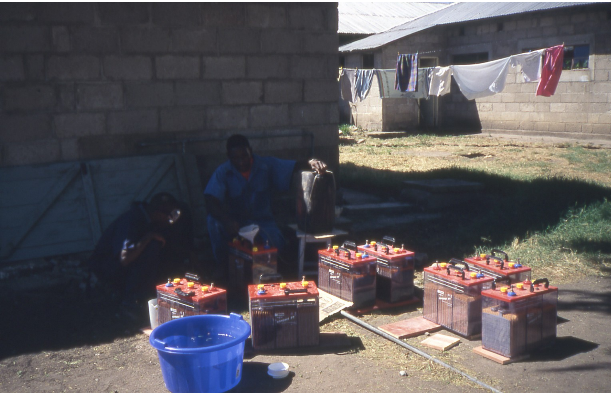
Putting acid in new batteries – note goggles, gloves, bowls of water, Wasso Hospital, Tanzania
