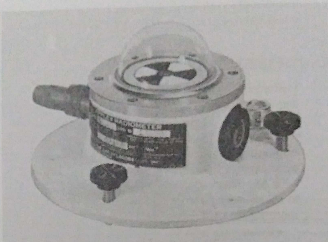
Figure 2.3.1 The Eppley black-and-white pyranometer. Courtesy of The Eppley Laboratory.
