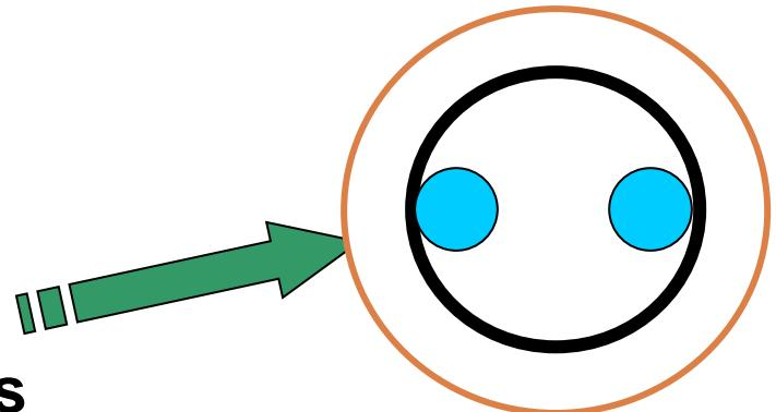
**No metal absorber plate is used. Vacuum is created in the interspace between the 2 glass tubes**
