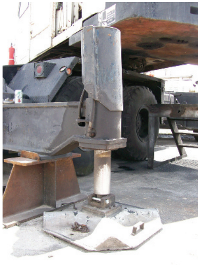
Cranes are often supported using bearing pads to give them stability. Care must be taken not to crush the supporting surface, due to the large bearing stress developed between the pad and the surface.
