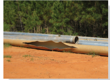
This thin-walled pipe was subjected to an excessive gas pressure that caused it to rupture in the circumferential or hoop direction. The stress in this direction is twice that in the axial direction as noted by Eqs. 8–1 and 8–2.
